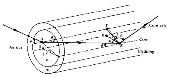
The ray path within the fiber core for a skew ray incident at an angle  $\theta$ s to the normal at the air—core interface.
